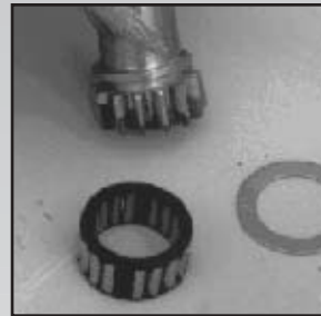
Clean all parts with solvent except 37857/37863.
